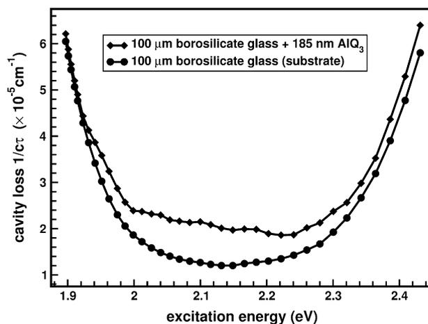
Fig. 3. Cavity loss spectra of the ringdown cavity with blank substrate (disks) and with  $\text{AlQ}_3$  covered substrate (diamonds) as a function of the excitation energy. The overall loss structure is due to the varying mirror reflectivity over the energy scan-range applied.
