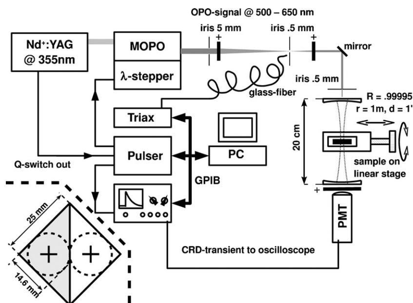
Fig. 1. Main figure: schematic of the CRD spectrometer setup used. Inset lower left: layout of the borosilicate glass substrate with one half blank and the other half covered with  $\text{AlQ}_3$ . Indicated are the areas on both halves available for irradiation.
