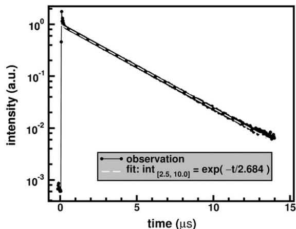
Fig. 2. Ringdown transient on a semi-log scale observed for 2.1 eV excitation energy of the cavity with the blank borosilicate glass substrate present. A least squares fit to the datapoints between 2.5 and 10  $\mu\text{s}$  yields a ringdown time of  $\tau = 2.684 \mu\text{s}$ .
