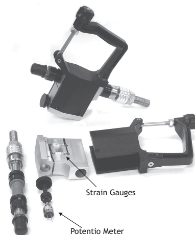
Figure 6.2. Oarlock sensor, including force and angle transducers.
