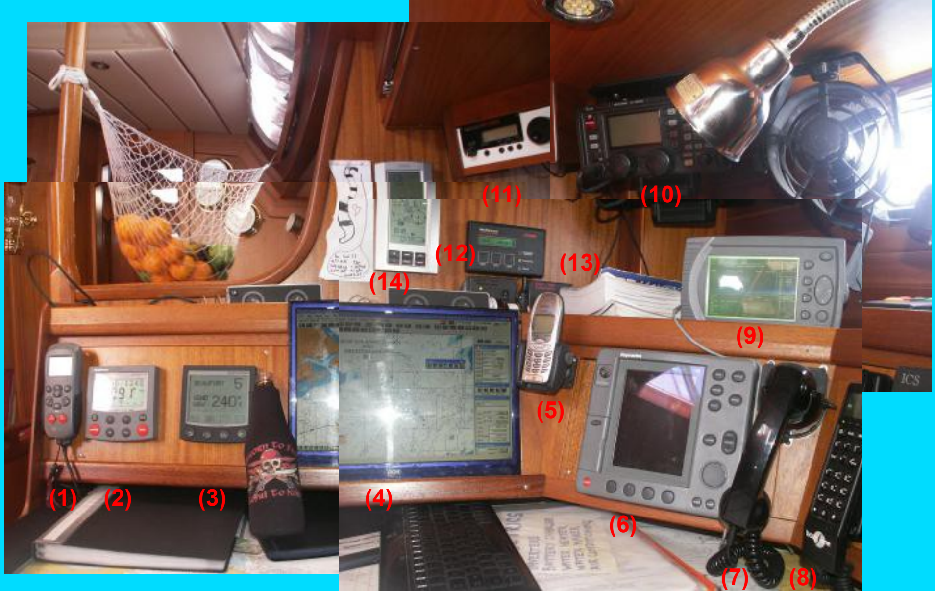
mosaic of navigation-corner with: (1) remote for autopilot, (2) autopilot console, (3) windforce and direction display, (4) navigation PC screen, (5) gsm, (6) radarscreen, (7) MF/HF handset, (8) inmarsat-satellite telephone, (9) AIS-transponder, (10) SSB (MF/HF) radio, (11) MF/HF-receiver, (12) barometer, (13) SeaMe radar-reflection enhancer, (14) home and kitchen weatherstation. Not visible: Navtex and VHF-radio.
